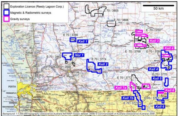
Bullamine Joint Venture tenements showing areas covered by the geophysical surveys underway. The magnetic and radiometric surveys are being flown at 50 metre flight line spacing, whilst the Falcon (gravity) surveys are at 200 metre flight line spacing.
