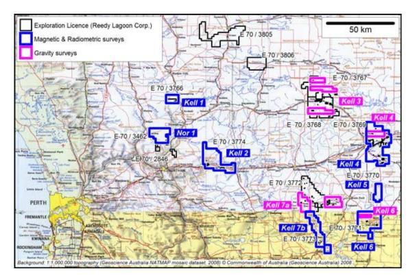
Bullamine Joint Venture tenements showing areas covered by the geophysical surveys completed. The magnetic and radiometric surveys are at 50 metre flight line spacing, whilst the Falcon (gravity) surveys are at 200 metre flight line spacing.
