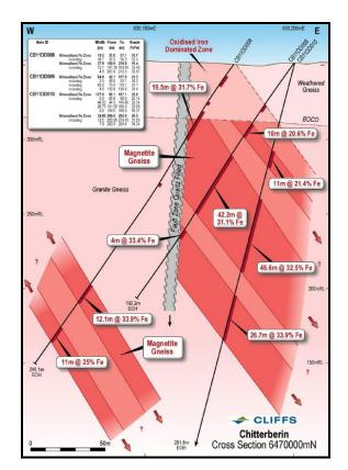
Chitterberin Prospect cross section (Bullamine JV, WA): Near surface mineralisation with true thickness between 30 to 100m.
