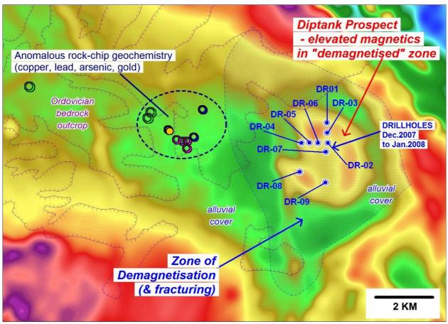
( Background image - total magnetic intensity, reduced to pole, Gaussian equalised )
