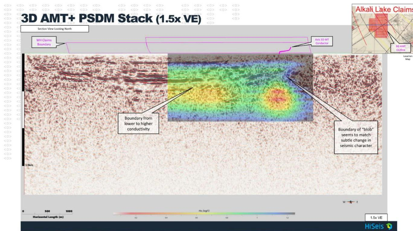
Figure 1. 2D Shallow Seismic Survey results superimposed on 3D AMT Survey Results (refer ASX [Release 14/10/2021](#))
