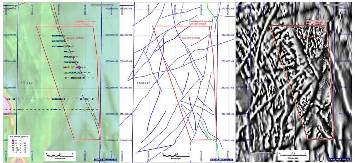
Figure 2. Lady Janet prospect. Gold in soil data shown over regional magnetics (TMI), LH panel; Structure interpreted using additional drone survey data, centre panel; processed drone survey magnetics (AGC), RH panel.
