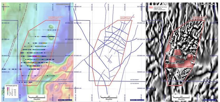
Figure 3. Windmills prospect. Gold in soil data shown over regional magnetics (TMI), LH panel; Structure interpreted using additional drone survey data, centre panel; processed drone survey magnetics (AGC) with areas precluded from survey shaded red, RH panel.
