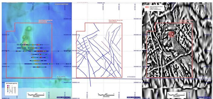
Figure 5. Zebra prospect. Gold in soil data shown over regional magnetics (TMI), LH panel; Structure interpreted using additional drone survey data, centre panel; processed drone survey magnetics (AGC) with area precluded from survey shaded red, RH panel.
