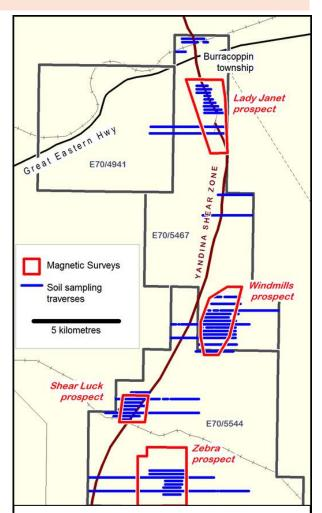
Figure 1. Magnetic survey areas are shown in outline over previously completed soil sample traverse lines at the Lady Janet, Windmills, Shear Luck and Zebra prospects.
