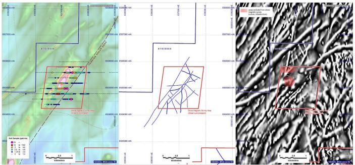
Figure 4. Shear Luck prospect. Gold in soil data shown over regional magnetics (TMI), LH panel; Structure interpreted using additional drone survey data, centre panel; processed drone survey magnetics (AGC) with areas precluded from survey shaded red, RH panel.
